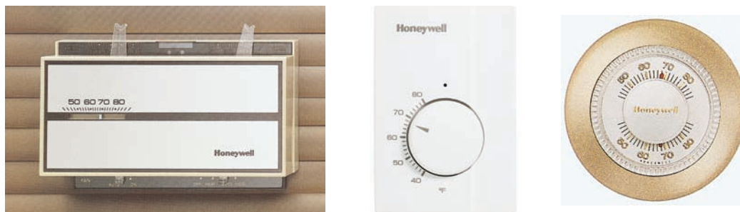
FIGURE 23-2 Thermostats for electric heating systems. A thermostat or other switching device that is marked with an “Off” position must open all ungrounded conductors of the circuit when turned to the “Off” position. Typical mounting height is 52 in. (1.3 m) to center. (Courtesy of Honeywell International Inc.)
