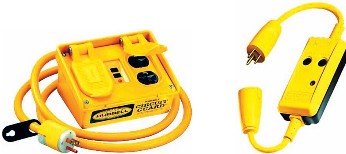
FIGURE 6-23 Cord-and-plug-connected “portable” GFCI devices are easy to carry around. They can be used anywhere when working with electrical tools and extension cords. These devices operate independently and are not dependent on whether the branch circuit is GFCI protected. These portable GFCI in-line cords are relatively inexpensive and should always be used when using portable electric tools. (Courtesy of Hubbell Lighting Outdoor & Industrial)
