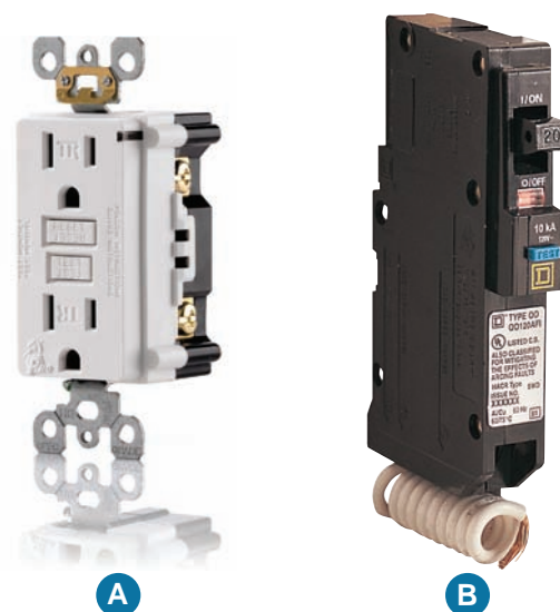
FIGURE 6-7 (A) A ground-fault circuit interrupter and tamper-resistant receptacle (courtesy of Leviton Manufacturing), and (B) a ground-fault circuit interrupter circuit breaker (Courtesy of Schneider Electric). The switching mechanism of a GFCI receptacle opens both the ungrounded “hot” conductor and the grounded conductor. The switching mechanism of a GFCI circuit breaker opens the ungrounded “hot” conductor only.
