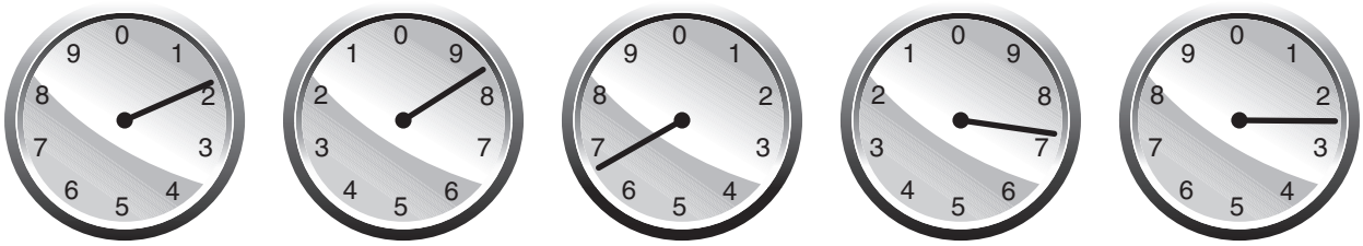
FIGURE 29-3 The reading of this five-dial meter is 18,672 kilowatt-hour. (Delmar/Cengage Learning)
