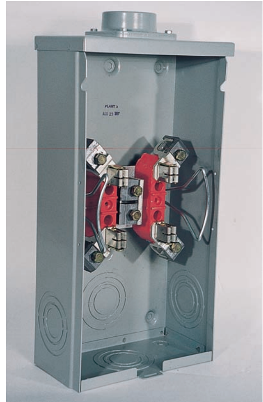
FIGURE 27-15 Typical residential self-contained meter socket. Combination meter socket/main breaker in one enclosure is also available. (Courtesy of Schneider Electric)
