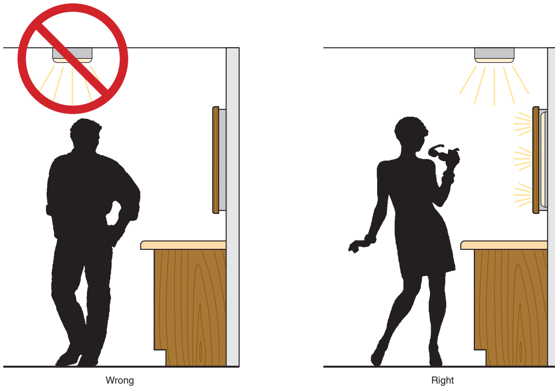
FIGURE 10-4 Positioning of bathroom luminaires. Note the wrong way and the right way to achieve proper lighting. (Delmar/Cengage Learning)
