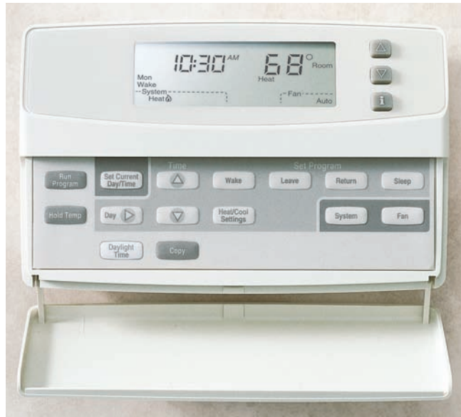
FIGURE 24-7 A digital electronic programmable thermostat that provides proper cycling of the heating system, resulting in comfort as well as energy savings. This type of thermostat, depending on the model, can be programmed to control temperature, time of operation, humidity, ventilation, filtration, circulation of air, and zone control. Installation and operational instructions are furnished with the thermostat. (Courtesy of Honeywell International Inc.)
