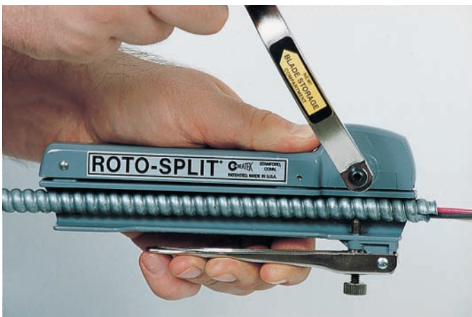
FIGURE 4-24 This is an example of a tool that precisely cuts the outer armor of armored cable, making it easy to remove the armor with a few turns of the handle. (Courtesy of Seatek Co., Inc.)
