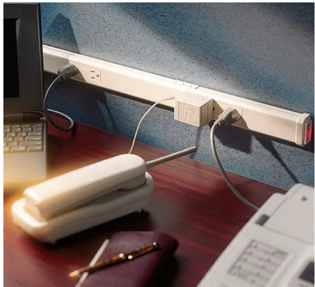
FIGURE 18-16 A typical metal multioutlet assembly. Multioutlet assemblies are permitted to be run through (not within) a dry partition when no outlets are located within the partition, and all exposed portions of the assembly can have the cover removed. Nonmetallic multioutlet assemblies are also available. (Courtesy of The Wiremold Company)
