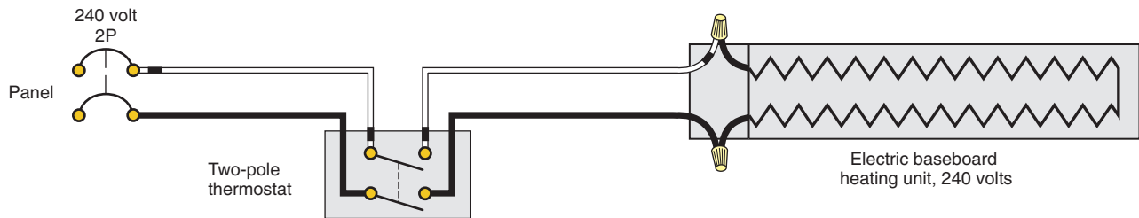
FIGURE 23-4 Wiring for a single electric baseboard heating unit. The thermostat is a line-voltage thermostat. See Figure 23-3 caption for color-coding requirements. (Delmar/Cengage Learning)
