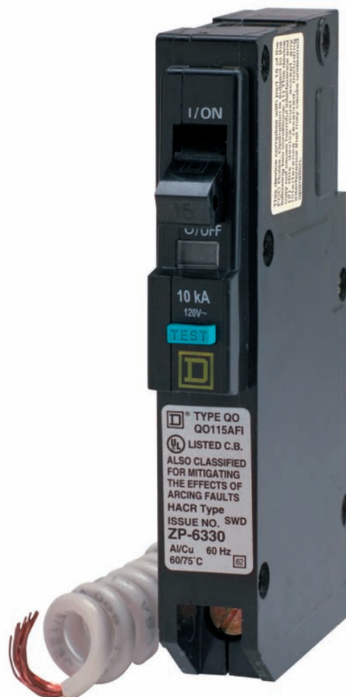
FIGURE 6-13 A listed combination-type arc-fault circuit-interrupter (AFCI) circuit breaker. (Courtesy of Schneider Electric)
