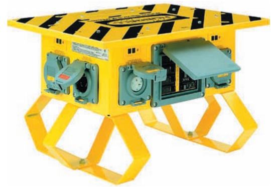
FIGURE 6-22 A temporary power box used on construction sites. This particular type is connected with a 50-ampere, 120/240-volt power cord. It has six 20-ampere, GFCI-protected, 125-volt receptacles plus additional 30-ampere and 50-ampere Twist-Lock receptacles. (Courtesy of Hubbell Lighting Outdoor & Industrial)
