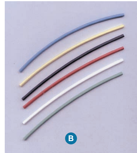
FIGURE 5-2 Shows a white conductor reidentified with black plastic electrical tape. (B) Shows an assortment of easy-to-use, 6-in.-long heat shrink tubing that is slid over the conductor to be reidentified, then shrunk tightly over the conductor by applying heat as specified in the instructions. (Delmar/Cengage Learning)
