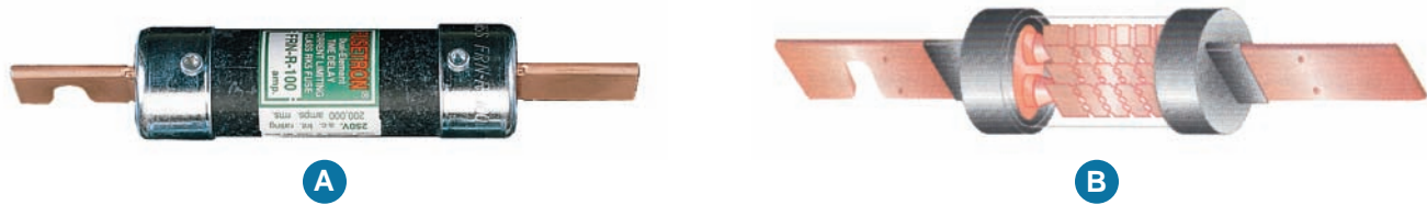
FIGURE 28-8 Cartridge-type dual-element fuse (A) is a 250-volt, 100-ampere fuse. The cutaway view in (B) shows the internal parts of the fuse. When this type of fuse has a rejection slot in the blades of 70–600-ampere sizes, or a rejection ring in the end ferrules of the 0–60-ampere sizes, it is a UL Class RK1 or RK5 fuse. (Courtesy of Cooper Bussmann)
