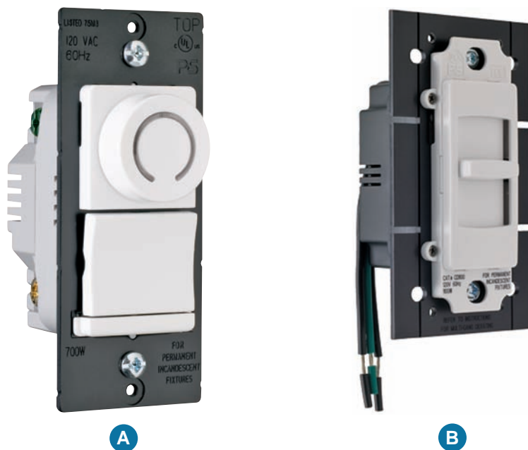
FIGURE 13-10 Some typical electronic dimmers. Both perform the same function of varying the voltage to the connected incandescent lamp load: (A) rotating knob; (B) slider knob. (Courtesy of Legrand/Pass & Seymour)
